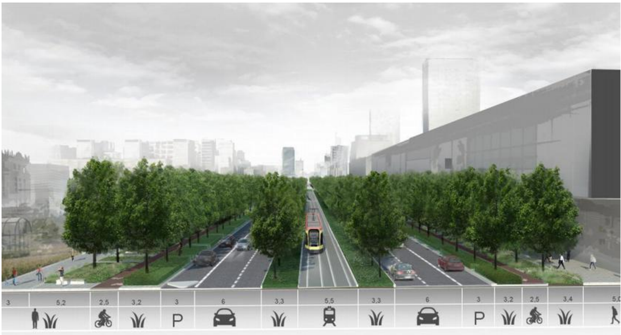
A vision of the proposed new profile for Marszałkowska avenue for the Public Roads Authority suggests planting four more rows of trees, shrinking the roadway to 4 narrow lanes (2+2 lanes) with longitudinal parking, two 2.5 m wide bike lanes and over 8 m sidewalks. Some of these features may however not be retained in the final project. © Architektura Krajobrazu
