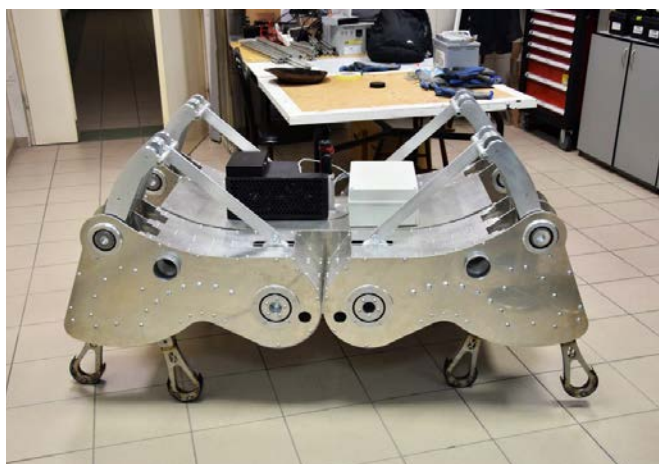
↑photo: Krab – autonomous walking robot developed by the students and employees of the Faculty of Mechanical Engineering.
