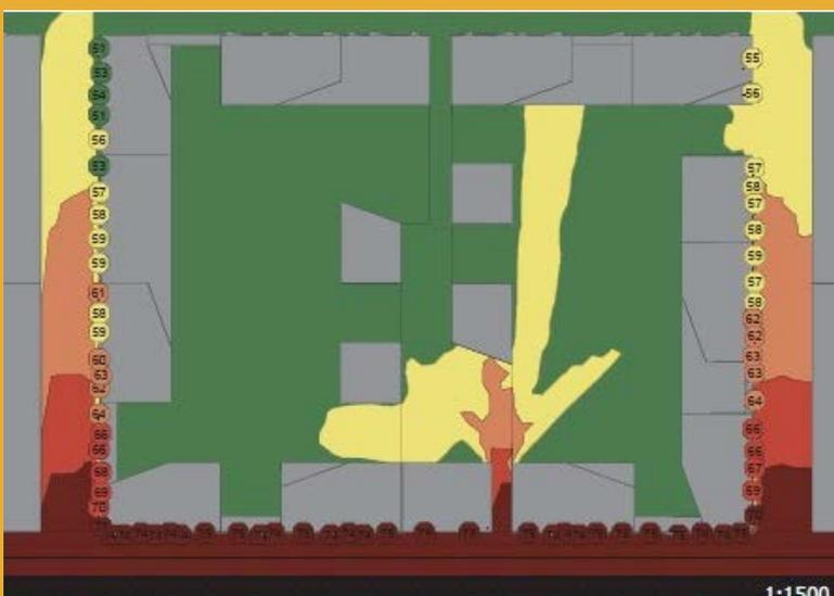
Noise simulation of a partly open housing block showing how the noise enters the courtyard with a 75,000 cars a day boulevard
