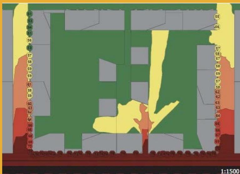
Noise simulation of a partly open housing block showing how the noise enters the courtyard with a 75,000 cars a day boulevard
