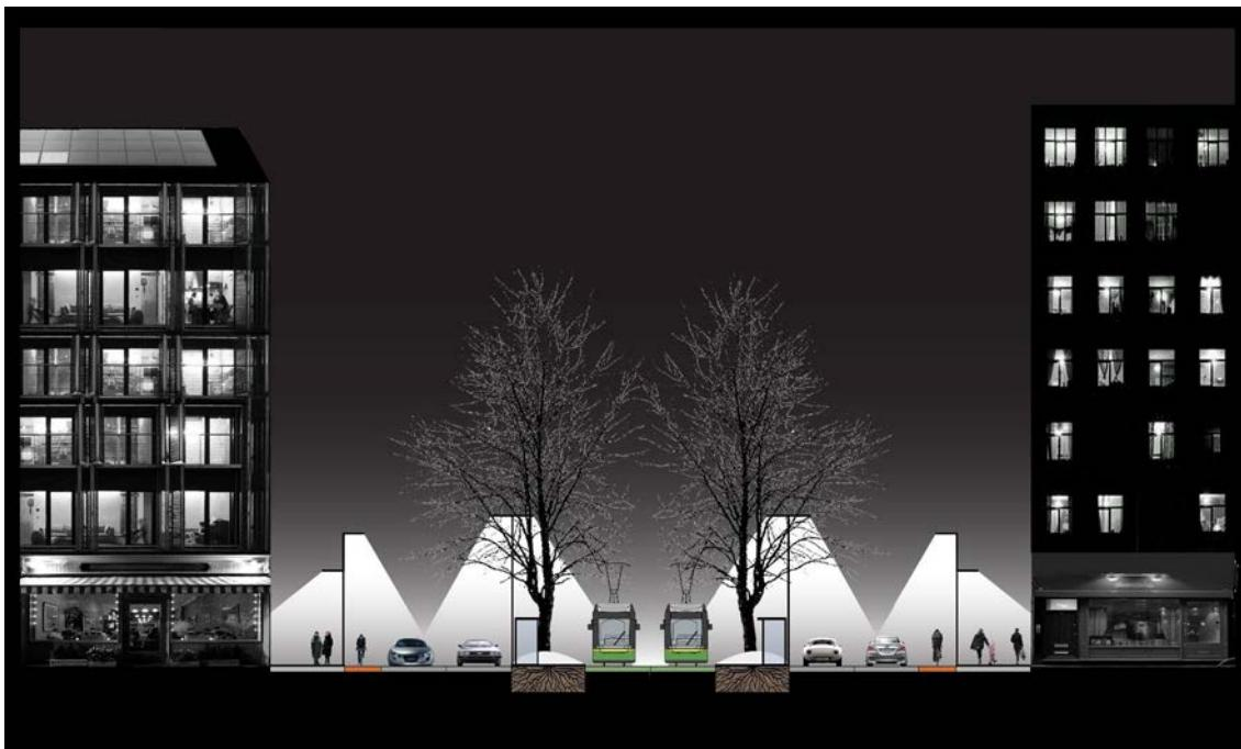
**A typical public space split for section of a 41 m tramway boulevard**
